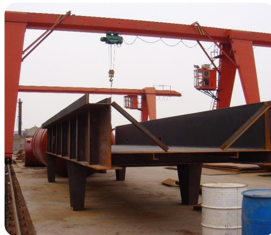
钢铁厂衬胶酸洗槽
